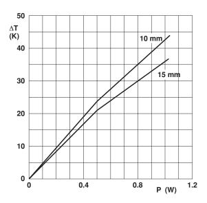
Temperature rise ( $\Delta T$ ) at the lead end (soldering point) as a function of dissipated power at various lead lengths after mounting.
