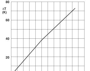
Hot-spot temperature rise  $(\Delta T)$  as a function of dissipated power.
