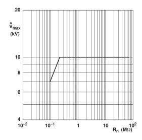
Maximum allowed peak pulse voltage in accordance with "IEC 60065 chapter 14.1"; 50 discharges from a 1 nF capacitor charged to  $\stackrel{\wedge}{V}_{max}$ ; 12 discharges/minute (drift  $\Delta$ R/R  $\leq$  2%).
