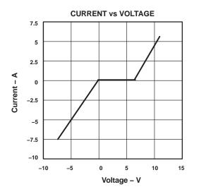
NOTE A: Typical current versus voltage curve was derived using the IEC 1.2/50-µs surge waveform.
