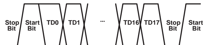
Figure 3. Serial Output Data Stream with Start and Stop Bit
