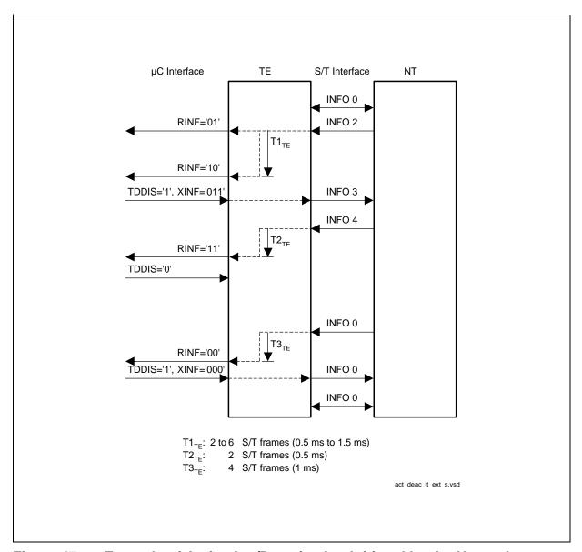
Figure 47 Example of Activation/Deactivation Initiated by the Network Termination (NT).
