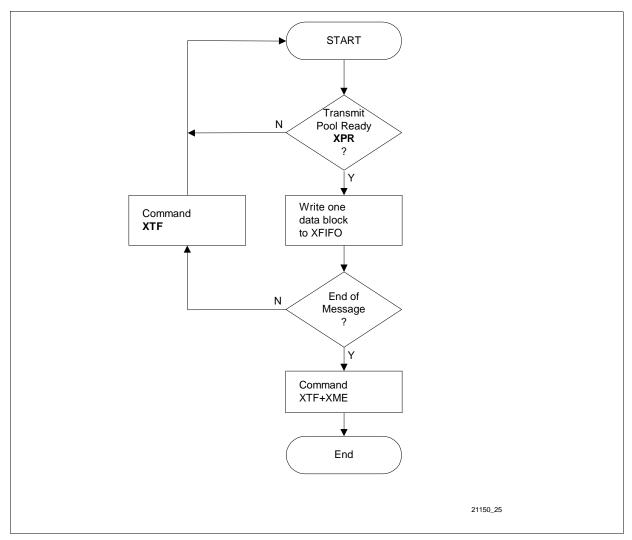
Figure 82 Data Transmission Procedure
