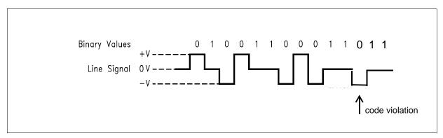
Figure 19 S/T -Interface Line Code
