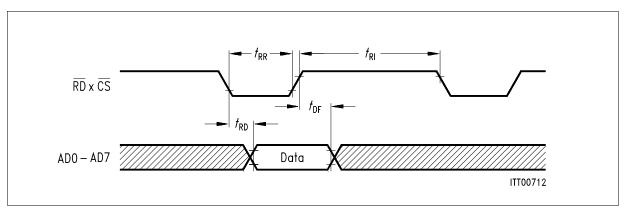
Figure 94 Microprocessor Read Cycle
