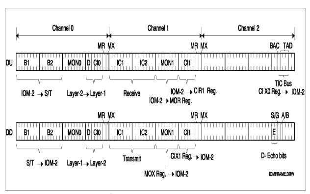
Figure 48 IOM®-2 Frame Structure in Terminal Mode
