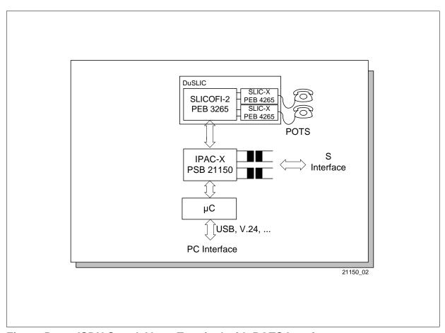
Figure 5 ISDN Stand-Alone Terminal with POTS Interface
