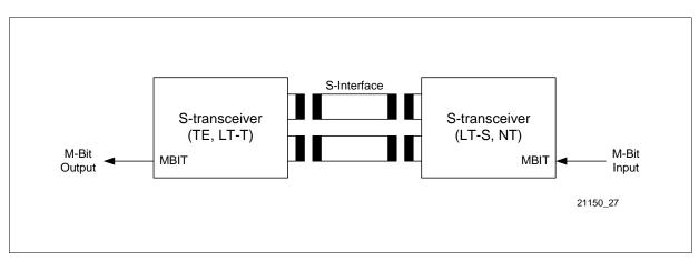
Figure 21 Multiframe Synchronization using the M-Bit
