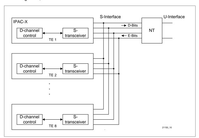
Figure 74 D-Channel Access Control on the S-Interface
