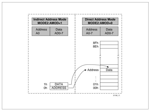
Figure 10 Direct/Indirect Register Address Mode
