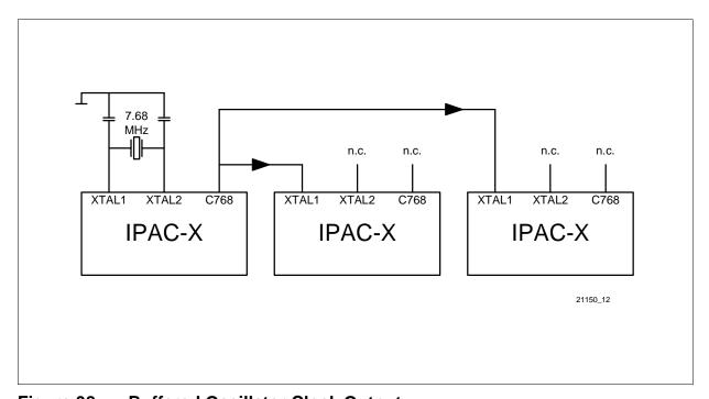
Figure 38 Buffered Oscillator Clock Output
