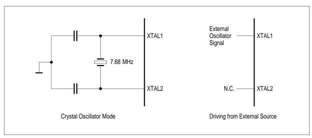
Figure 88 Oscillator Circuits
