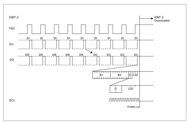
Figure 76 Deactivation of the IOM-2 Interface
