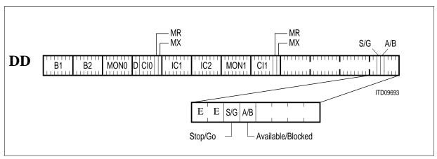
Figure 73 Structure of Last Octet of Ch2 on DD
