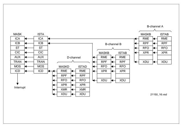
Figure 85 Interrupt Status Registers of the HDLC Controllers
