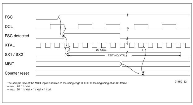
Figure 101 Sampling Time in LT-S/NT Mode (M-Bit Input)
