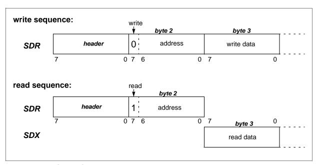
Figure 9 Serial Control Interface Timing
