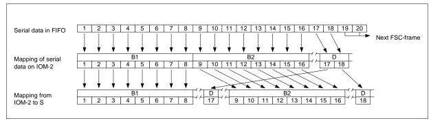
Figure 61 Mapping of Bits from IOM-2 to S
