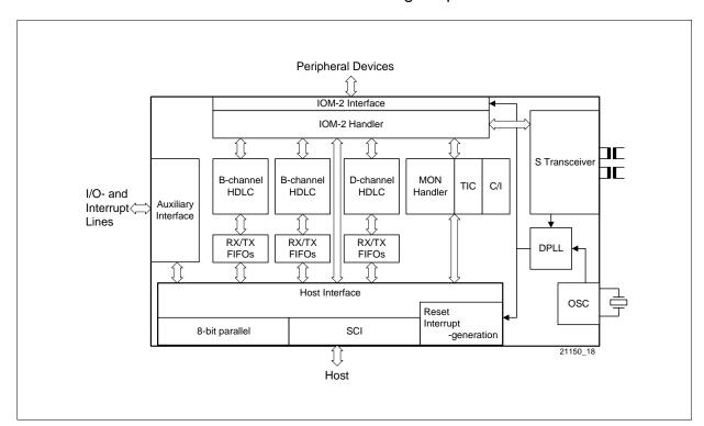
Figure 7 Functional Block Diagram of the IPAC-X
