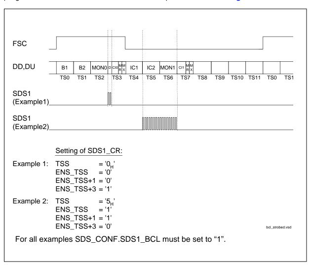
Figure 63 Strobed IOM-2 Bit Clock. Register SDS\_CONF Programmed to 01<sub>H</sub>
