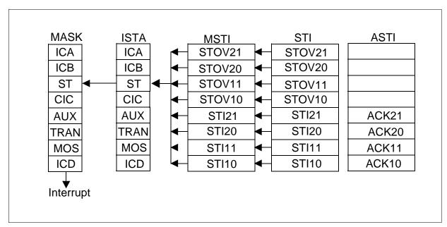
Figure 56 Interrupt Structure of the Synchronous Data Transfer
