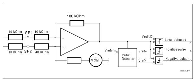
Figure 30 Equivalent Internal Circuit of the Receiver Stage
