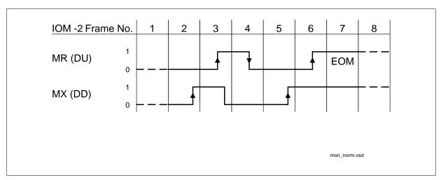
Figure 68 Monitor Channel, Normal End of Transmission
