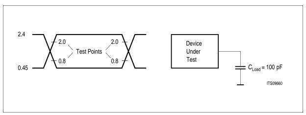
Figure 89 Input/Output Waveform for AC Tests
