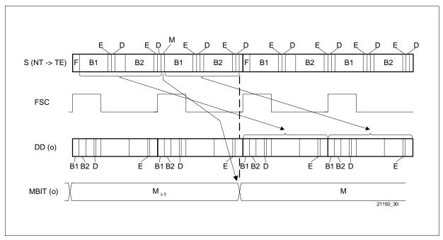
Figure 24 Frame Relationship in TE / LT-T mode (M-Bit output)
