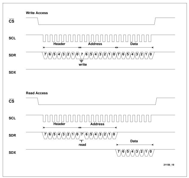
Figure 8 Serial Control Interface Timing
