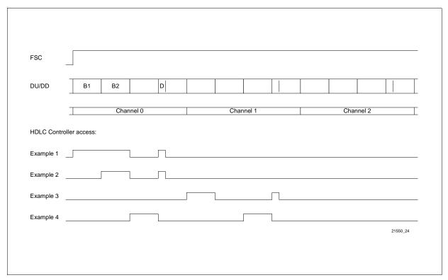
Figure 59 Examples for HDLC Controller Access
