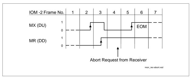
Figure 66 Monitor Channel, Transmission Abort Requested by the Receiver
