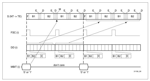
Figure 23 Frame Relationship in LT-S / NT mode (M-Bit input)
