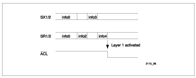
Figure 16 ACL Indication of Activated Layer 1
