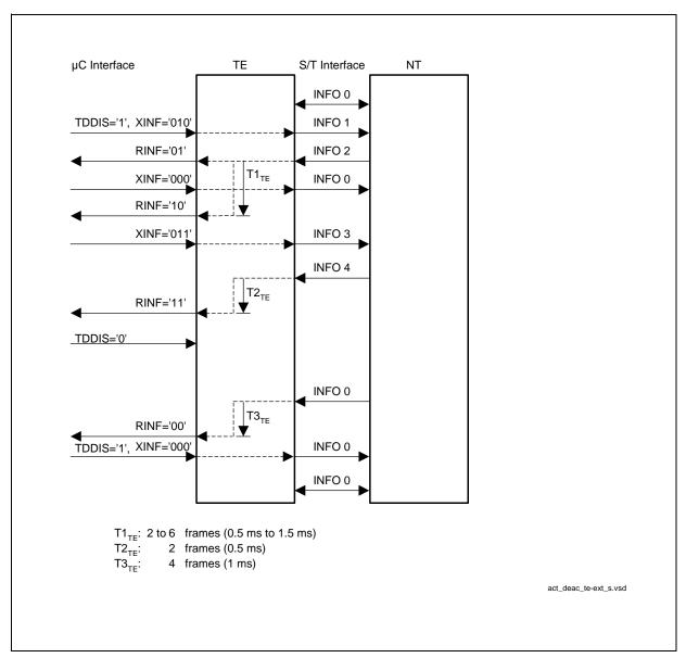
Figure 46 Example of Activation/Deactivation initiated by the Terminal (TE).
