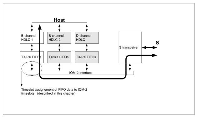
Figure 58 Timeslot Assignment on IOM-2
