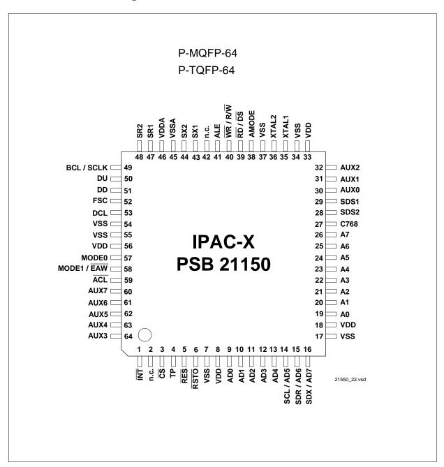
Figure 6 Pin Configuration of the IPAC-X
