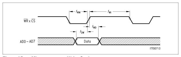
Figure 95 Microprocessor Write Cycle
