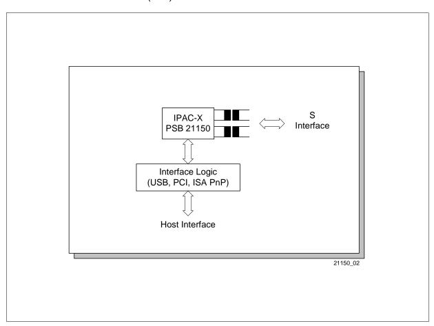
Figure 2 ISDN PC Adapter Card for S Interface
