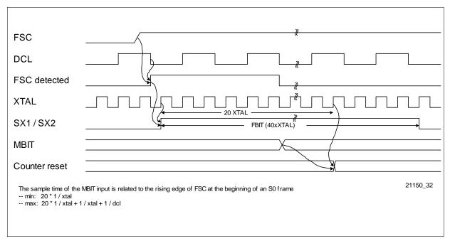
Figure 22 Sampling Time in LT-S / NT mode (M-Bit input)
