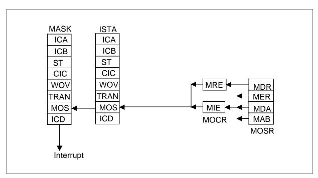
Figure 69 MONITOR Interrupt Structure
