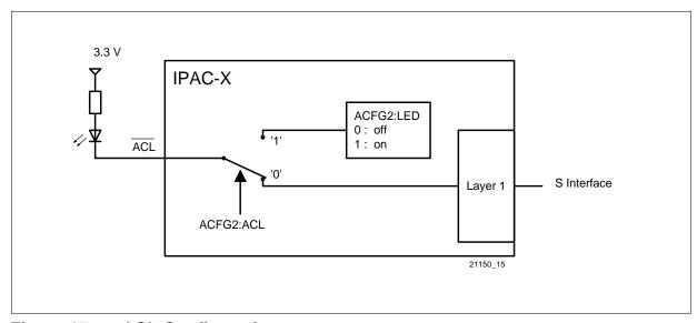
Figure 17 ACL Configuration
