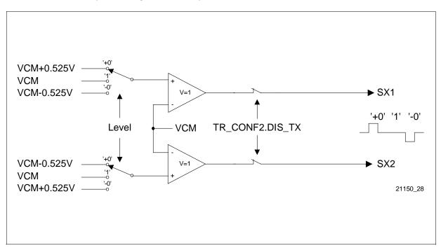
Figure 29 Equivalent Internal Circuit of the Transmitter Stage
