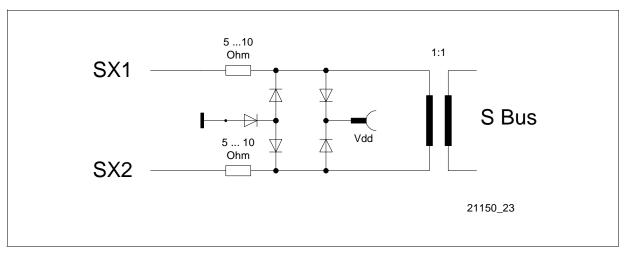
Figure 32 External Circuitry for Transmitter
