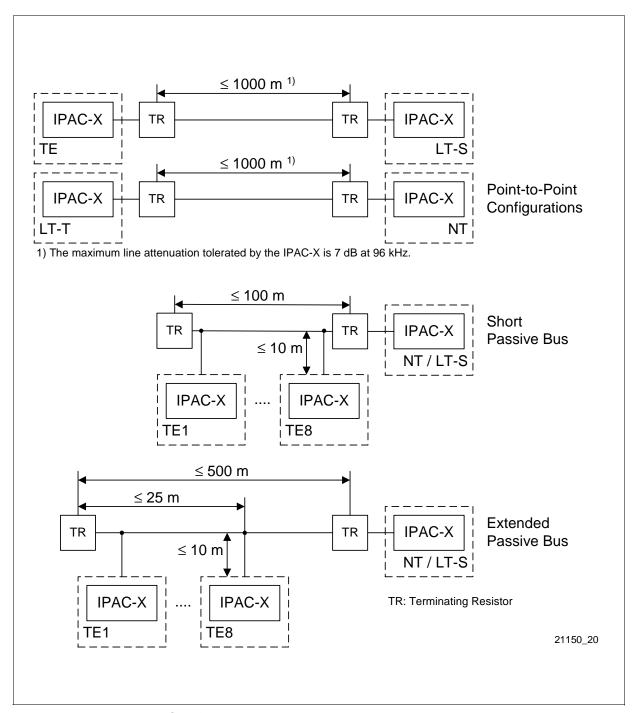
Figure 18 Wiring Configurations in User Premises
