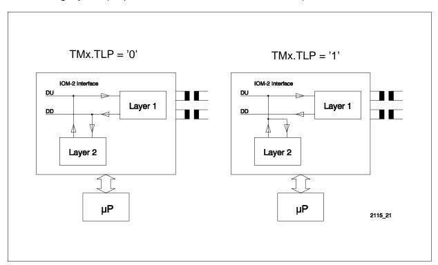
Figure 86 Layer 2 Test Loops
