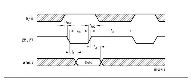
Figure 98 Microprocessor Read Timing
