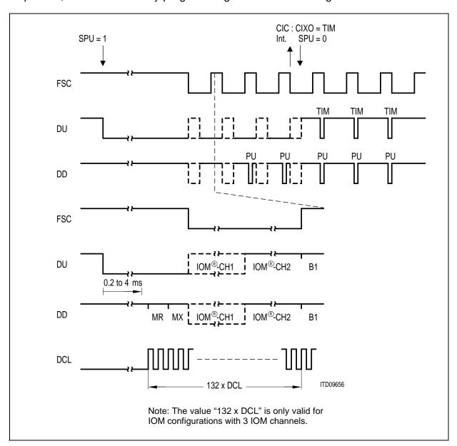
Figure 77 Activation of the IOM-2 interface
