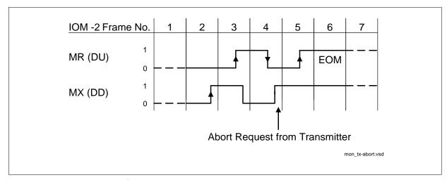
Figure 67 Monitor Channel, Transmission Abort Requested by the Transmitter
