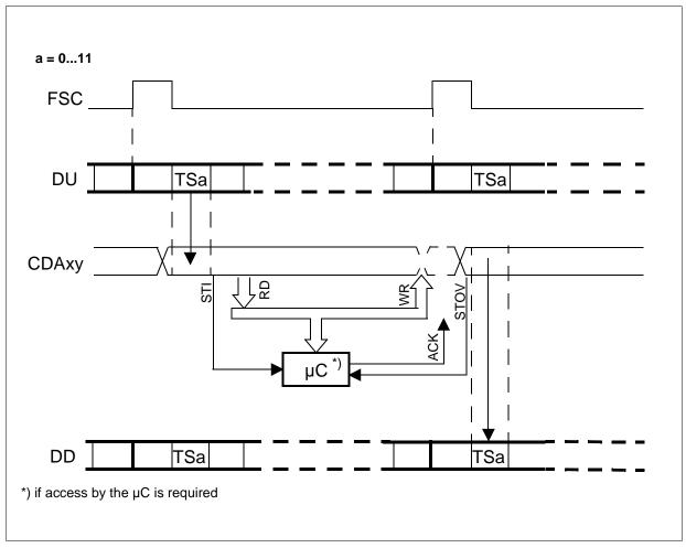
Figure 53 Data Access when Looping TSa from DU to DD
