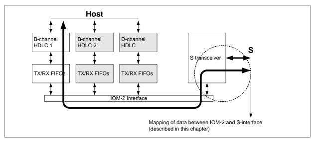
Figure 60 Timeslot Assignment on S
