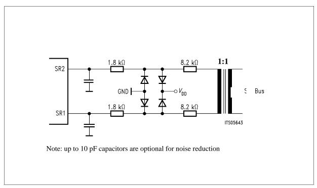
Figure 33 External Circuitry for Symmetrical Receivers
