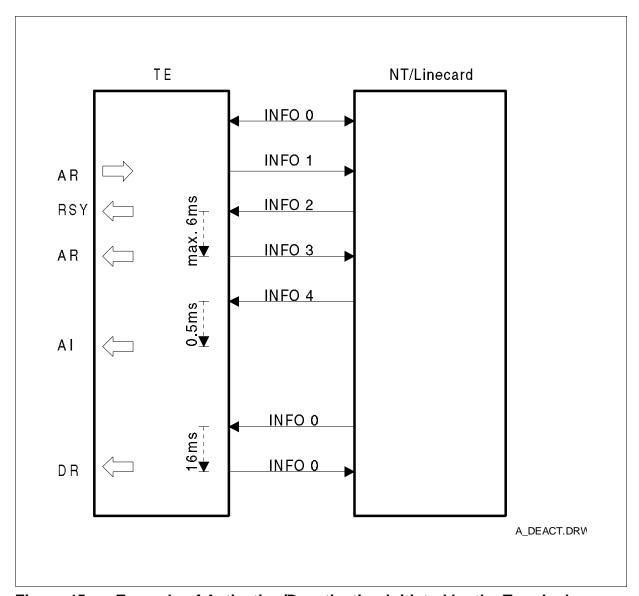
Figure 45 Example of Activation/Deactivation Initiated by the Terminal
