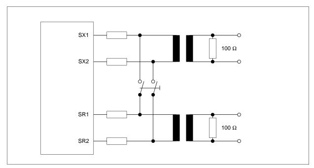
Figure 35 External Loop at the S/T-Interface
