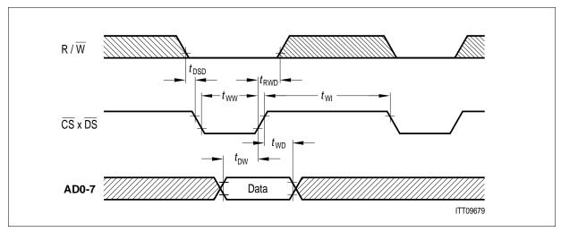
Figure 99 Microprocessor Write Cycle
