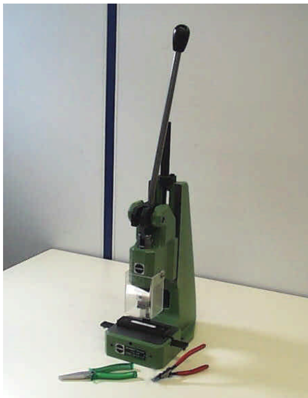
Figure 17 -- Connector Removal tooling HM2Y350
