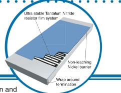
The IRC TaNFilm® PFC chip resistor series provides the high precision and ultra stable performance of our Tantalum Nitride resistive film system in 0603, 0805, 1206, 1505, 2010 and 2512 sizes. The unique characteristics of the passivated Tantalum Nitride film insure long term life stability and stability in most environments.
