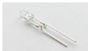
6 3 mm, Sicke/3 mm, crimping
