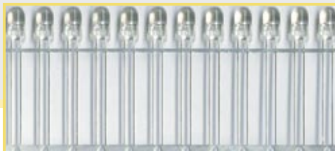
LEDs im Leadframe/ LED in a leadframe
