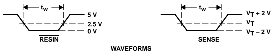
Figure 2. Input Pulse Definition
