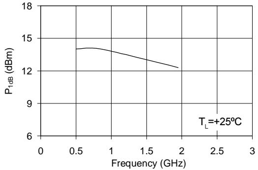
**Typical RF Performance Over Temperature ( Bias:  $V_D = 3.2$  V,  $I_D = 45$  mA (Typ.) )**
