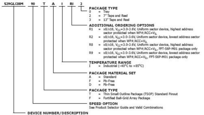
S29GL128M 128 Megabit Page-Mode Flash Memory Manufactured using 0.23 um MirrorBit™ Process Technology, 3.0 Volt-only Read, Program, and Erase
