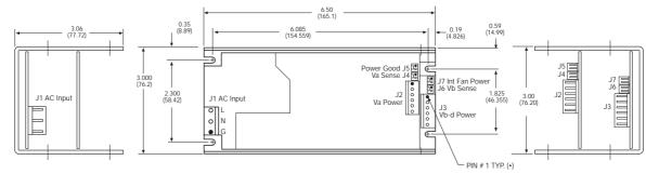
Va is the first output Vb is the second output Vc is the third output Vd is the fourth output.
