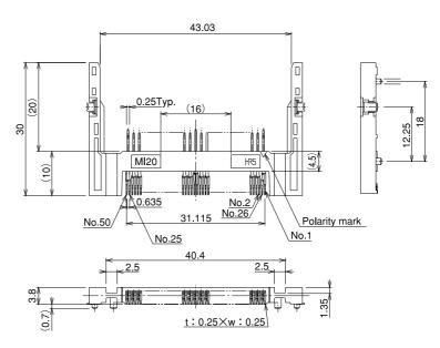
Note 1: Coplanarity of all surface mount terminals and components is 0.1.
