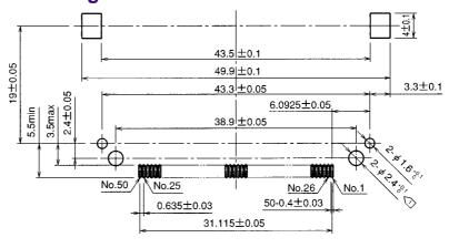
Note  $\boxed{1}$  The holes  $(2-\emptyset 2.4^{+0.1}_{0})$  illustrated in the figure are only required when screws are used for fastening.
