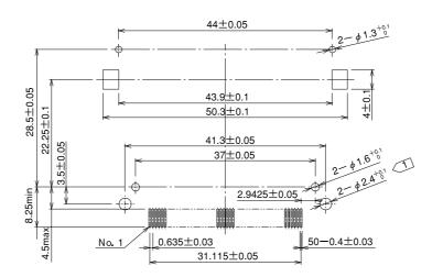
Note  $\boxed{1}$  The holes  $(2-02.4^{+0.1}_{0})$  illustrated in the figure are only required when screws are used for fastening.
