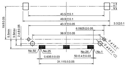
Note  $\boxed{1}$  The holes  $(2-0.4^{+0.1})$  illustrated in the figure are only required when screws are used for fastening.
