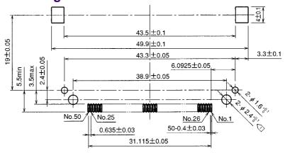
Note  $\boxed{1}$  The holes  $(2-\sqrt[9]{2}.4^{+0.1})$  illustrated in the figure are only required when screws are used for fastening.
