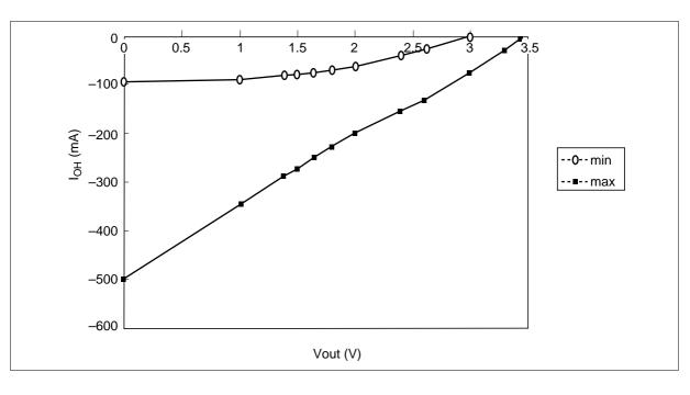
**DC Characteristics** (Ta = 0 to 70°C,  $V_{CC}$ ,  $V_{CC}$ Q = 3.3 V  $\pm$  0.3 V,  $V_{SS}$ ,  $V_{SS}$ Q = 0 V) (HM5264165)
