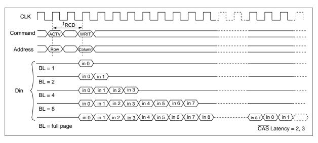
**2. Single write:** A single write operation is enabled by setting OPCODE (A9, A8) to (1, 0). In a single write operation, data is only written to the column address (AY0 to AY7; HM5264165, AY0 to AY8; HM5264805, AY0 to AY9; HM5264405) and the bank select address (A12/A13) specified by the write command set cycle without regard to the burst length setting. (The latency of data input is 0 clock).
