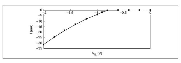
Minimum  $V_{IH}$  Clamp Current (referred to  $V_{CC}$ )
