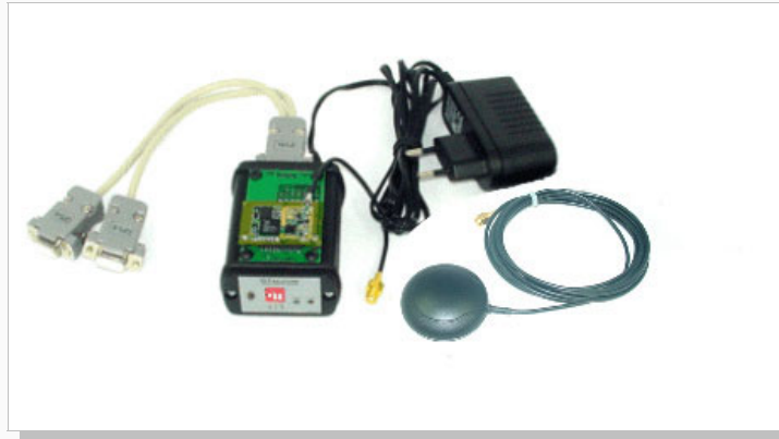
Figure 18: Evaluation board with connected JP13 GPS receiver.
