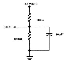
\* INCLUDING SCOPE AND JIG CAPACITANCE
