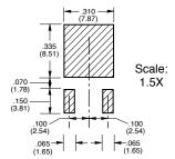
**Soldering Note:** During surface mount soldering the soldering temperature profile must not cause the metal tab of this device to exceed 220°C.
