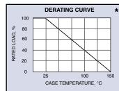
The case temperature is to be used for purposes of establishing the maximum applied power. See Derating Curve. The case temperature measurement is made on the metal mounting tab against the molded body. Derate appropriately for the ambient temperature range, the thermal resistance of the mounting surface, and the temperature limitations of the adjacent materials (such as glass epoxy).
