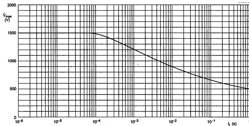
Fig. 18 Pulse on regular basis; maximum permissible peak pulse voltage ( V_{max} ) as a function of pulse duration ( t_i )
